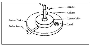
Figure 10. Mattress Firmness Test Fixture.
