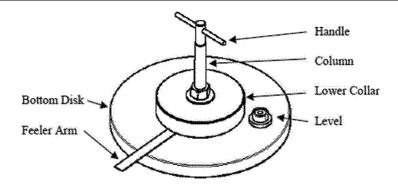
(iv) 7.13.1.2 Included on the fixture, but not overhanging the footprint, shall be a linear level that is positioned on a plane parallel to the bar, and in a direction parallel to the bar.
