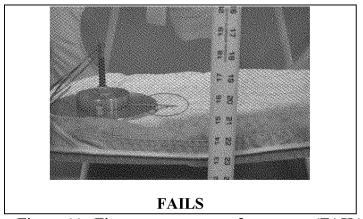
Figure 11. Firmness test on a soft mattress (FAIL)
