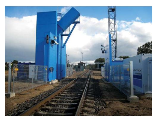
7.82 A further example of a Nuctech scanner with an energy level ranging from 1.5MeV to 6MeV that is used for "inspecting cars, cargo containers, empty containers, container trucks at seaports, border crossings, airports" is shown below<sup>98</sup>:
